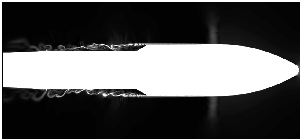
Figure 3.4: Instantaneous schlieren over a launcher shrinkage
