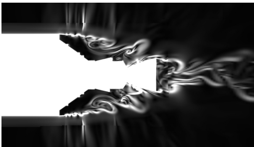
Figure 5.7: Instantaneous Schlieren around Ariane 5 launcher in the plane without boosters.
