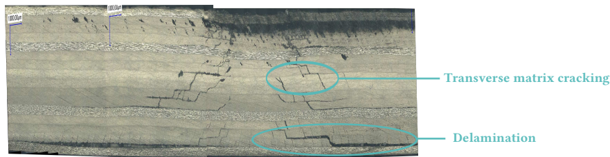
Figure 3.2 – Damage modes in unidirectional carbon/epoxy composite.
