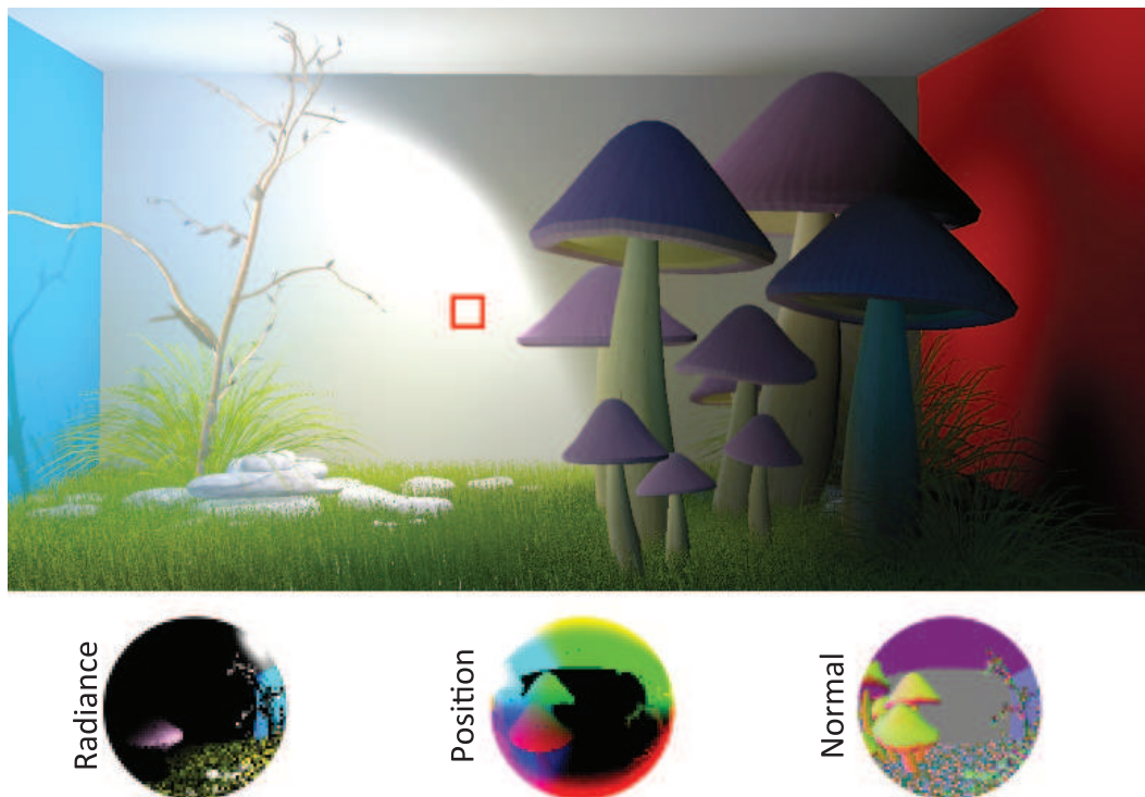
Figure 3.18: Top: Point-Based GI in a scene (700 k triangles, 1 M points) rendered at a resolution of 1024 \times 1024 with 4096 views in 29 ms. Bottom: Radiance, position and normal for one indirect lighting view (red box).
