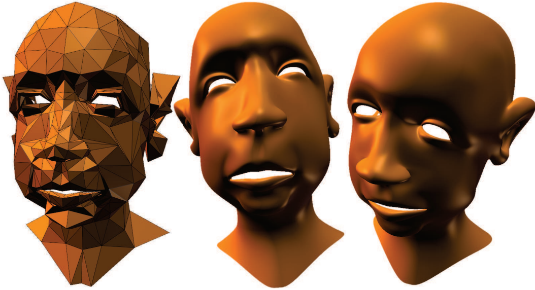
Figure 2.6: Left: Input coarse mesh. Middle and right: real-time adaptive subdivision of the animated input mesh using our method.
