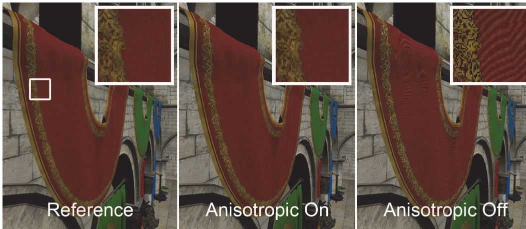
Figure 4.9: Left: reference using full 3 \times 3 supersampling with anisotropic filtering, middle: our approach with anisotropic filtering, right: our approach without anisotropic filtering.
