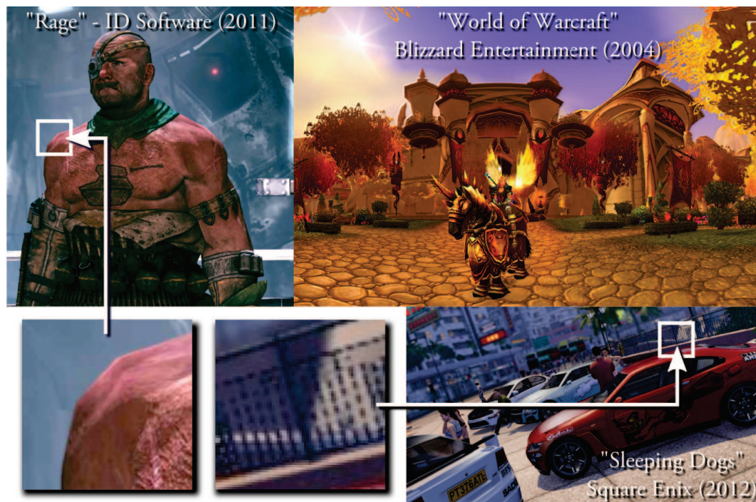
Figure 1.7: Screenshots from various games. Although high quality texture maps improve image and shading quality, creating smooth and nicely looking geometry is still a challenging problem, especially for animated characters. This is most obvious when silhouettes are undertessellated (top left image with closeup) and a trained eye can often differentiate between local tessellation schemes and nicer subdivision surfaces. Top right: High quality global lighting effects are still difficult to achieve in real time and often low quality solutions are used. This results in pictures that often look unnatural due to simplified lighting calculations that avoid the simulation of complex but important interactions of light with the scene. The bottom right picture with closeup reveals aliasing artifacts due to the low number of samples per pixel that were used. As a result, the elements of the fence seem disconnected.
