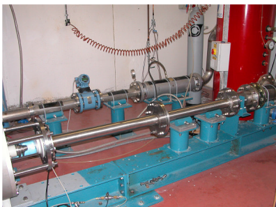
FIGURE 1.16 Banc d'essai Cavitating Pump Rotordynamic Test Facility [26] FIGURE 1.17 Inducteur sur Cavitating Pump Rotordynamic Test Facility [26]
