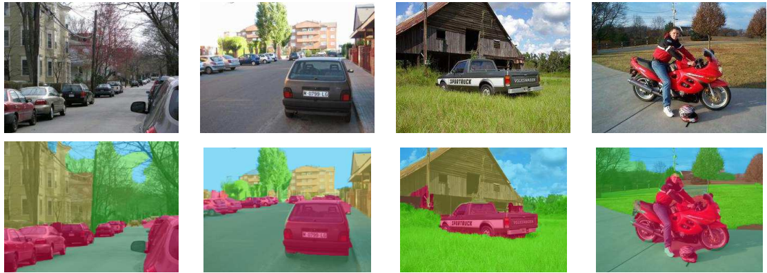
Figure 2.8: More Scene Parsing Results - More results using our multiscale convolutional network and a flat CRF on the Stanford Background Dataset.
