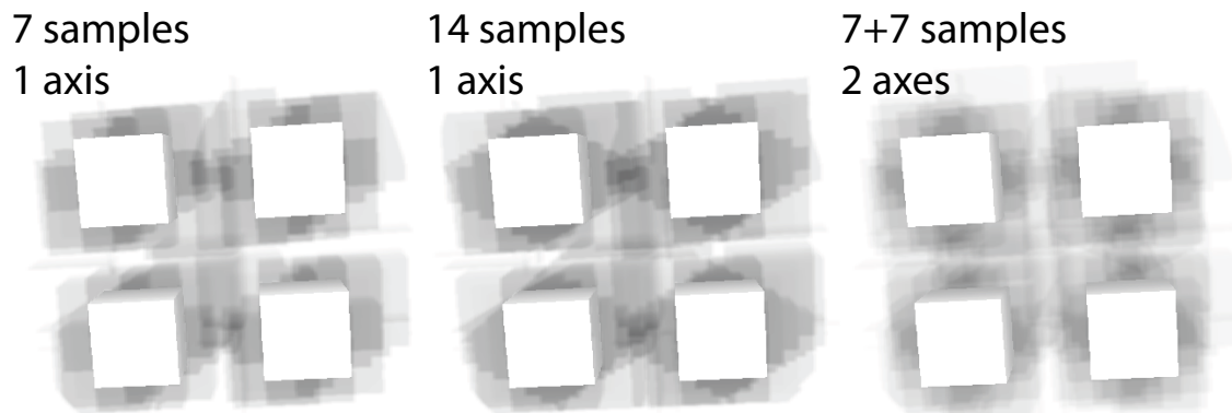
Figure 3.9: One axis does not provide enough information (left), even when using the same number of samples which leads to the same cost (middle), the result is inferior to a two-axis separation (right).
