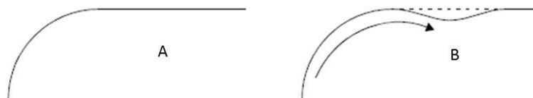
Figure 3.5: If the radius meets a straight line (A), the transition area appears hollow (B, exaggerated)
