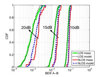
Figure 6-6: Comparison of the BER A-B computed over both the measurements and the model, for SNR=10, 15 and 20 dB.
