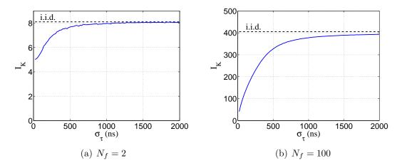
Figure 3-12: Variation of  $I_K$  with the RMS delay spread for  $\Delta \tau = 20$  ns.
