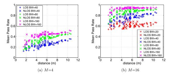
Figure 6-13: Mean pass rate as a function of the distance for 5.4 GHz and for frequency variability.
