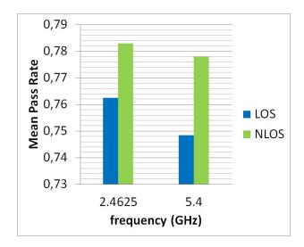
Figure 6-14: Mean pass rate exploiting frequency variability for  $BW=40~\mathrm{MHz}$  and M=16.
