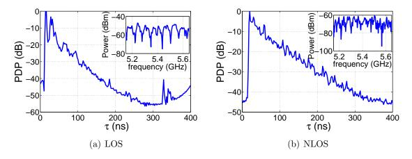
Figure 6-11: Examples of PDPs and channel transfer functions.
