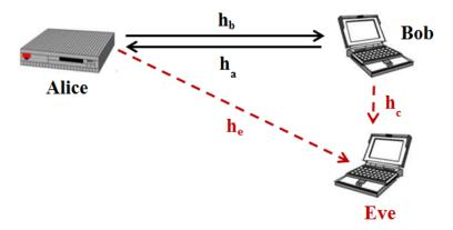
Figure 3-1: The terminals' propagation channels involved in the SKG scheme.
