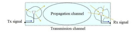
Figure 2-2: Transmission vs. propagation channel.
