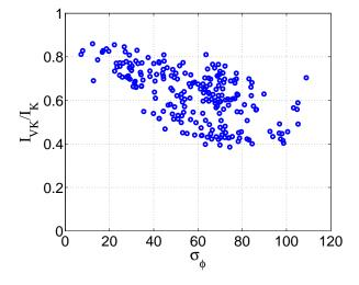
Figure 5-13:  $I_{VK}/I_K$  as a function of the angular spread, for  $N_f=1$  and  $d=0.1\lambda$ .
