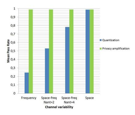
Figure 7-4: Mean pass rates before and after privacy amplification, for SKSM.
