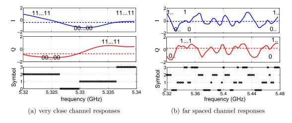
Figure 6-15: Example illustrating SKG from channel responses, for M=4.
