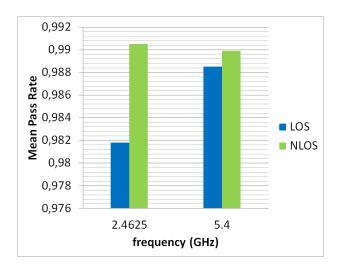
Figure 6-10: Mean pass rate exploiting spatial variability with respect to LOS/NLOS and for N = 128.
