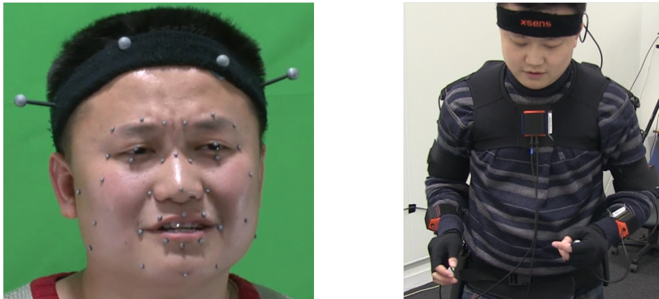
Figure 1.4: Actors equipped with motion capture technology. The left image shows the actor with motion capture sensors on his face. The right image shows the actor with motion capture sensors on his body.
