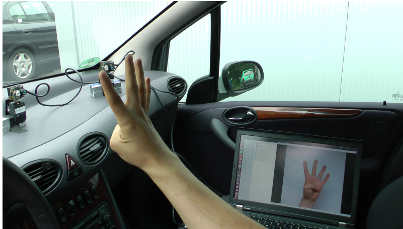
Figure 6.1: The initial system setup with two ToF sensors mounted to the front console.
