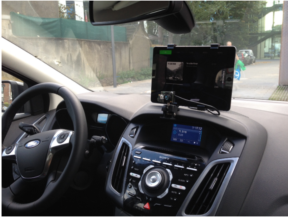
Figure 6.2: Complete system: sensor, laptop and tablet mounted to the front console visualizing the infotainment system. The main improvement for this system lies in the reduction to one camera only and, on the algorithmic side, in the novel ML methods introduced.
