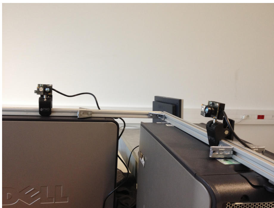
Figure 4.1: The recording setup for the multi-sensor database. Both sensors are aligned in a perpendicular angle to each other at a distance of approx. 49.5cm.
