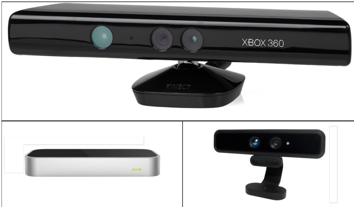
Figure 1.8: The Microsoft Kinect Sensor (top). The Leap Motion Controller (bottom left). The SoftKinetic Cam (bottom right). Source: Wikipedia.
