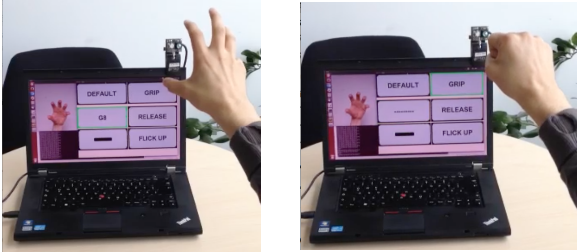
Figure 6.3: Demo setup: The user performs the grabbing gesture defined by the starting pose 'h' (left) and the ending pose 'f' (right) (cf. Figure 4.2 for notations)
