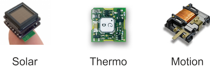
Figure 2.2: Ambient energy harvesting devices.
