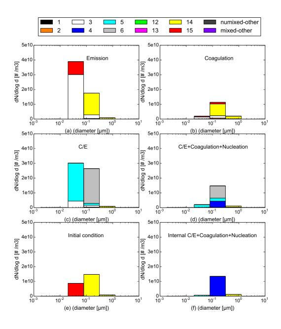
Figure 2.9: Result number distributions of externally-mixed particles as a function of particle diameter for the different chemical compositions for 6 different simulation scenarios: (a) Emission only; (b) Emission+Coagulation; (c) Emission+C/E; (d) Emission+Coagulation+C/E+nucleation; (e) Initial Condition; (f) Internal mixing result.
