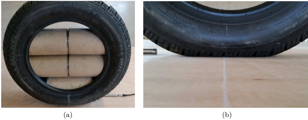
Figure 5.15: (a) The load of five concrete cylinders; (b) The contact zone between the tire and the road.
