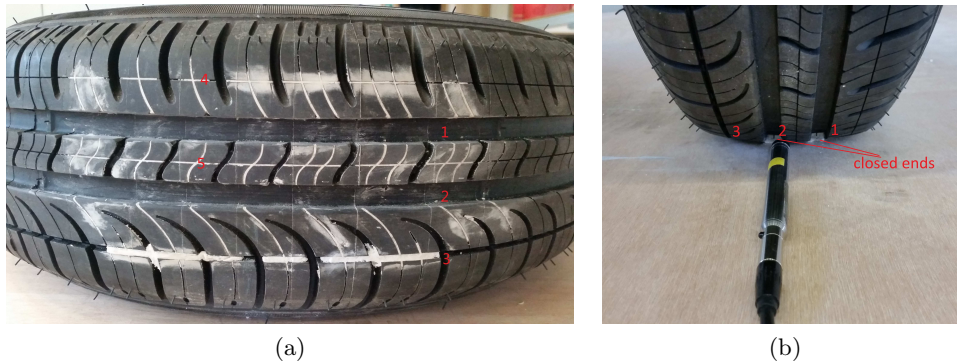
Figure 5.14: (a) Tire with an open network; (b) Tire with a closed network.
