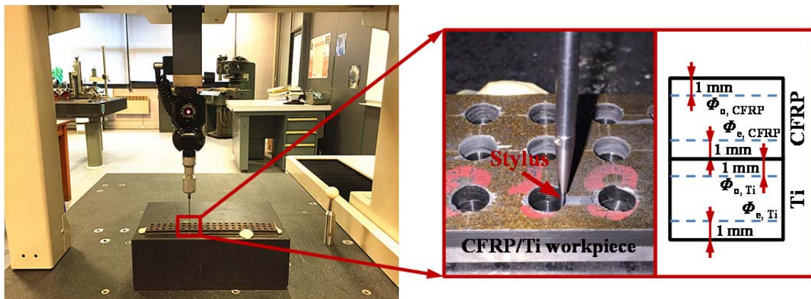
Figure 3.10. Photograph showing the process setup of hole dimensional feature measurement.
