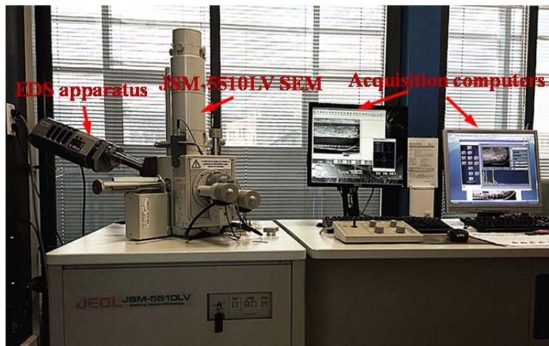
**Figure 3.11.** Photograph showing the used JSM-5510LV type scanning electron microscope (SEM).
