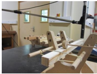
Figure 23 Samples placement on BING bending vibration method
