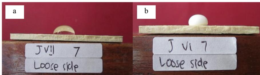
Figure 12 Contact angle of water (a) and PVAc as adhesive (b) on jabon veneers' loose side
