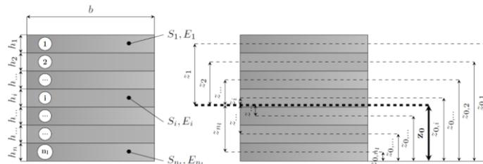
Figure 44 Geometrical and mechanical properties of LVL in a specimen cross-section
