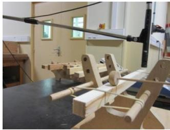
Figure 23 Samples placement on BING bending vibration method
