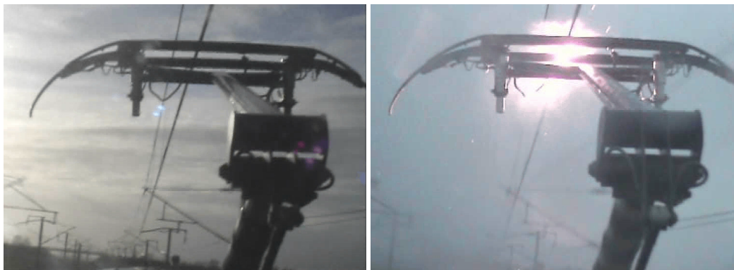
Figure 1.27: Good (left) and bad (right) current collection quality under the same catenary type for different weathers
