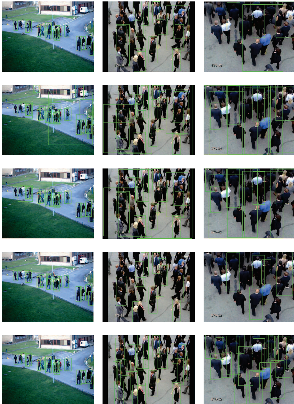
Figure 6.3: Exemplary visual results show how a crowd-sensitive threshold increases the detection performance compared to the baseline method while the proposed algorithm using an additional correction filter enhances the results further: (a) baseline algorithm at \tau_{min} , (b) baseline algorithm at \tau_{max} , (c) dynamically chosen \tau , (d) filtered detections (e) proposed method using dynamically chosen \tau and correction filter according to aspect ratio and perceived height. From Top to bottom: Frames from PETS 2009, UCF 879, and INRIA 879-38_I. For PETS and UCF, the proposed method generates more accurate detections and less clutter compared to the baseline method. Results for INRIA are also visibly better, but due to the camera view the effect of the correction filter is small.
