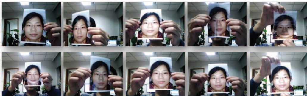
Figure 3.3: Different photo-attacks are shown from column (1) to column (5): (1) move the photo horizontally, vertically, back and front; (2) rotate the photo in depth along the vertical axis; (3) the same as (2) but along the horizontal axis; (4) bend the photo inward and outward along the vertical axis; (5) the same as (4) but along the horizontal axis. Figure is taken from [131].
