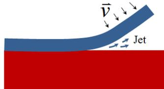
**Fig. 1.3** – Under proper impact velocity conditions a jet stream appear that cleans the contact zone.
