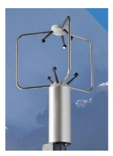
Figure 2.5 – 3D ultrasonic anemometer
