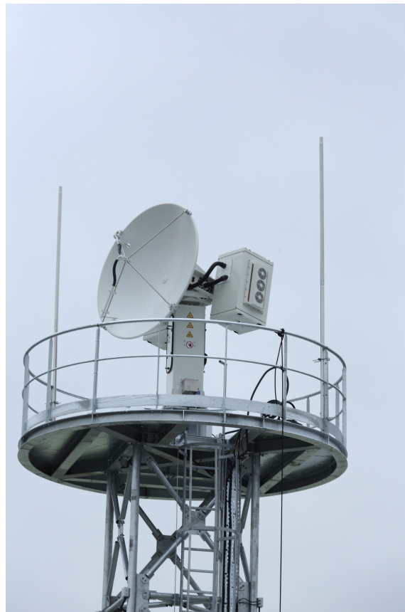
Figure 2.24: The new X-band polarimetric radar installed in the framework of RainGain project. © Rosa Vicari /HM&Co - ENPC
