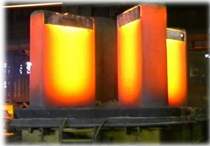
Fig.2. 1 – An illustrative figure presenting casting products (of several meters size) for which heterogeneities in compositions and structures are originated from microscopic processes that are then manifested at the system scale through advective mechanism
