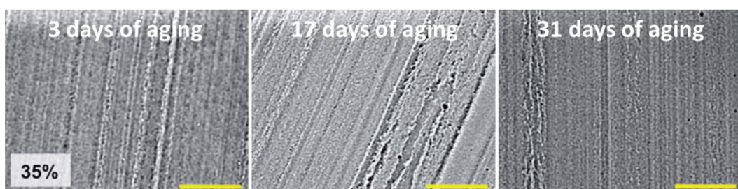
Figure 18 Micrographs of aged PVA hydrogels (35 wt% of PVA). Scale bar is 80 \mu\text{m} . 44
