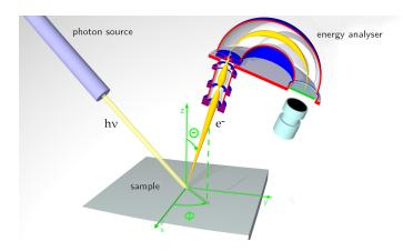
Figure 1.2: A schematic representation of an angle-resolved photoemission spectroscopy (ARPES) experiment taken from [26]. Besides the energy of the photoelectron, its angle is also measured in ARPES.
