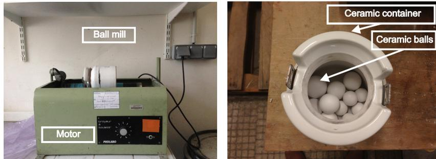
Figure 2.2: Ball mill used for the present work, consisting in a motor, a ceramic container, and ceramic balls.
