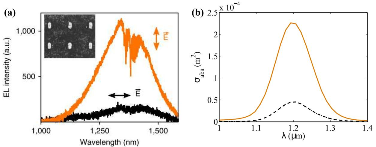
**Figure 6.9:** (a) The experimental electroluminescence results are presented for both light polarizations as a function of the wavelength for a setup with nanorods. Light polarized along the long axis of the nanorods gives more electroluminescence signal than light polarized along the short axis. Courtesy of Quynh Le-Van. (b) Numerical results of the calculation of the absorption cross section for quantum dots on top of a single nanorod with dimensions  $170 \times 50 \times 50 \text{ nm}^3$ .
