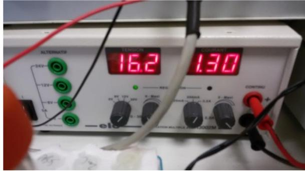
**FIGURE 4.13:** Electrical generator voltage is set to 16.2 V.
