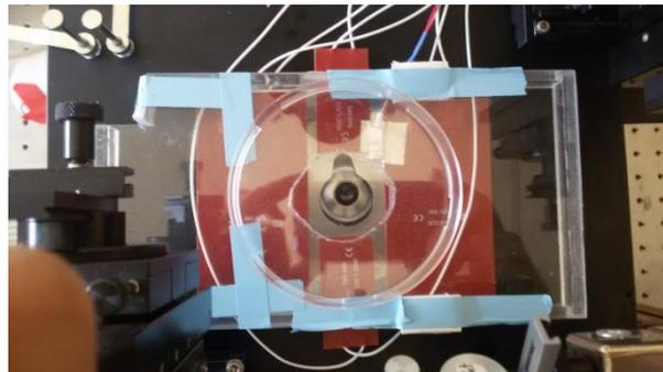
**FIGURE 4.12:** Layout of the experiment system with the lid and a thermocouple inside.
