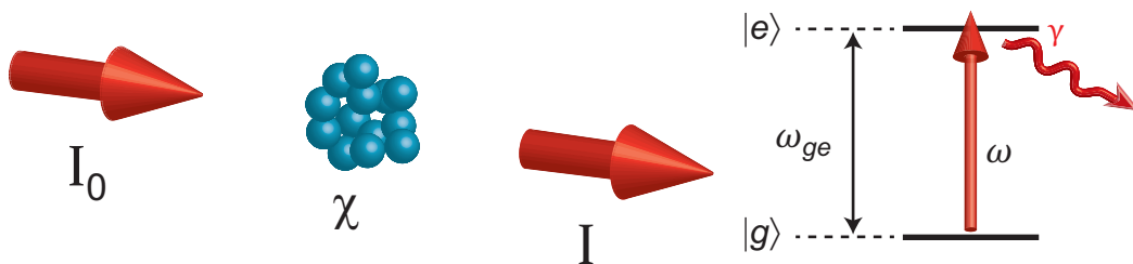
Figure 2.1: Two-level excitation scheme: Each atom is considered as a two-level system with ground state ‘g’ and excited state ‘e’. An optical beam with intensity I_0 is incident on the atomic media with frequency \omega , and we denote the susceptibility of the atoms as \chi . The energy difference between the two levels is denoted by \omega_{ge} .
