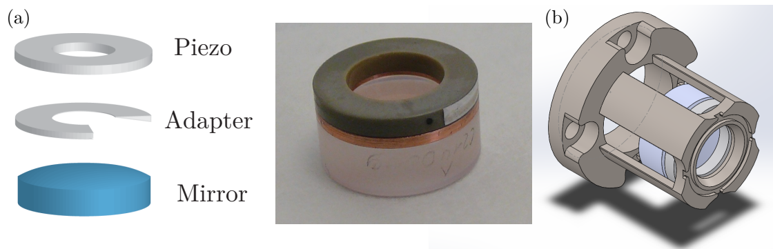
Figure 9.4: Configuration of the bottom mirror: (a) To minimize any fluctuations, the mirror and the piezo are glued using a triangular ring adapter to maximize the surface contact. A non-conducting glue is used to minimize any potential contacts between the electrodes of piezo and other surfaces. (b) Bottom mirror holder: A single piece was designed without any springs.
