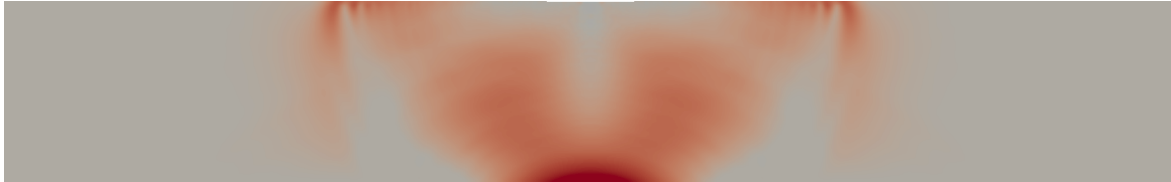
Figure 4.68 – The biggest eigenvalue of the stress tensor at t = 1.6 \times 10^{-4} s ranging from less than -7 MPa (blue) to more than 3 MPa (red). The compressive area is localized on the upper surface just under the impactor
