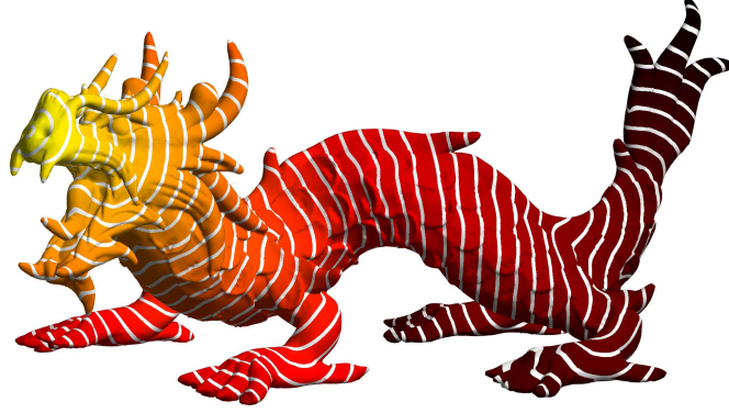
Figure 3.2 – Isolines of the geodesic distance, computed with the spectral method [34].
