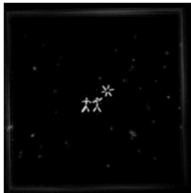
Figure 1.13: Reconstruction of the diffraction pattern represented on figure 1.12 [1]
