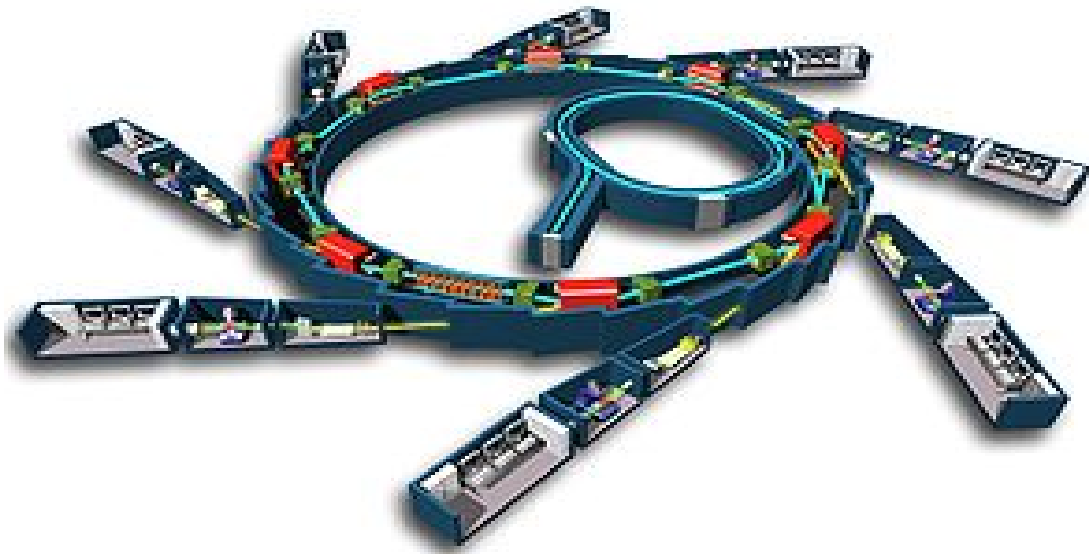
Figure 1.4: Scheme of principle of a standard synchrotron.
