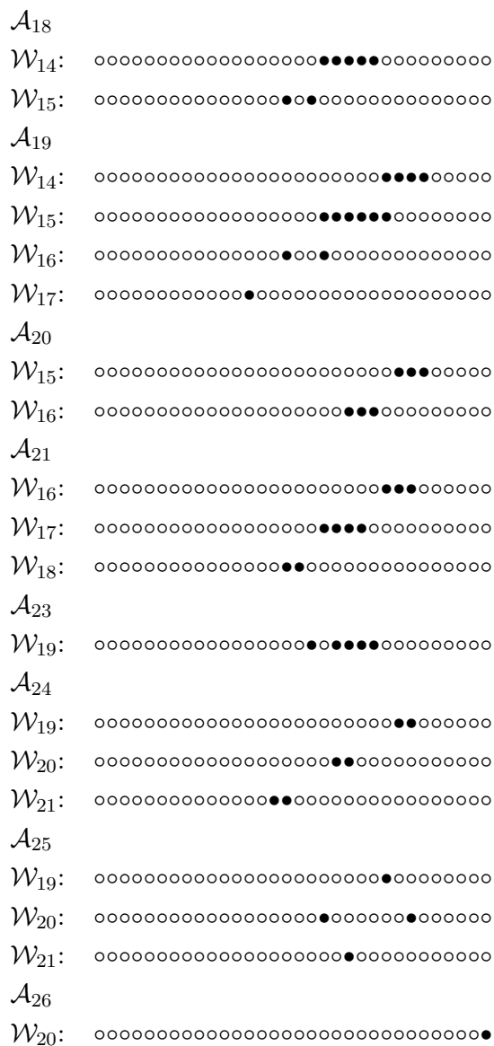
Figure 10.9 – The fifty-one neutral bits regrouped by the first state where they start to interact. A “•” represents the presence of a neutral bit, and a “o” the absence thereof. The LSB position is the rightmost one.
