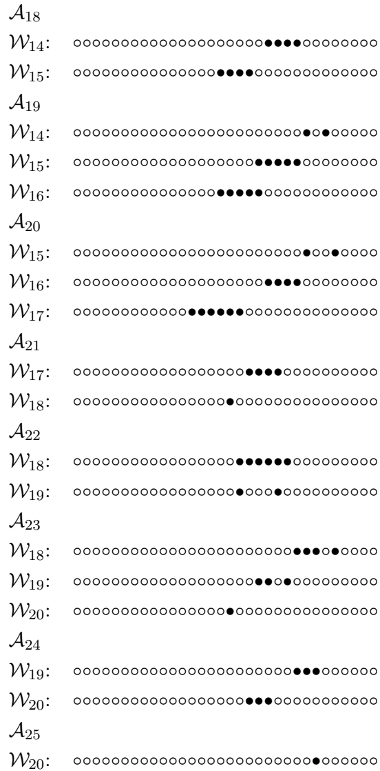
Figure 10.17 – The sixty neutral bits regrouped by the first state where they start to interact. A “●” represents the presence of a neutral bit, and a “○” the absence thereof. The LSB position is the rightmost one.
