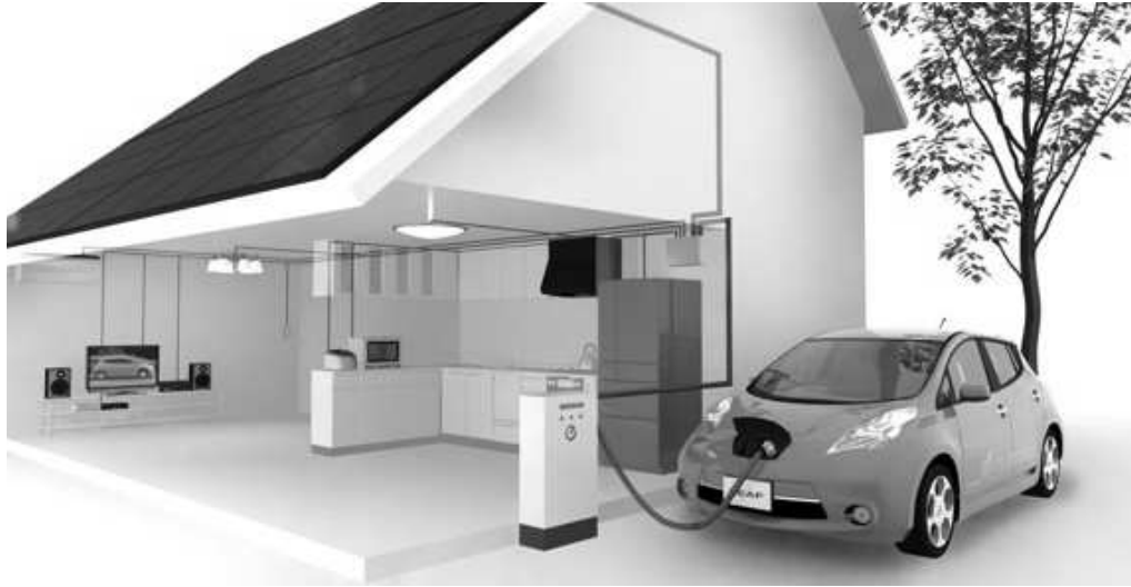
Figure 1.8: Vehicle-to-Home concept from Nissan motor corporation.
