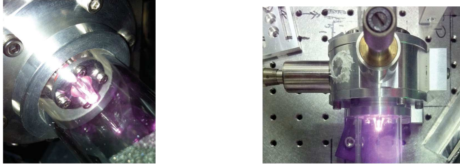
Figure 7.14 – Pictures of the glass-cone filter in the focus of the 10 mJ beam.
