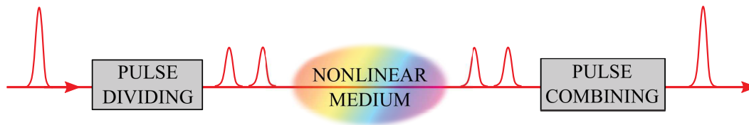
Figure 8.1 – Principle of optical multiplexing.
