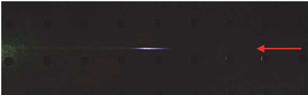
Figure 9.3 – Picture of the \approx 2 cm long filament. The direction of the incident laser pulses is indicated in red.
