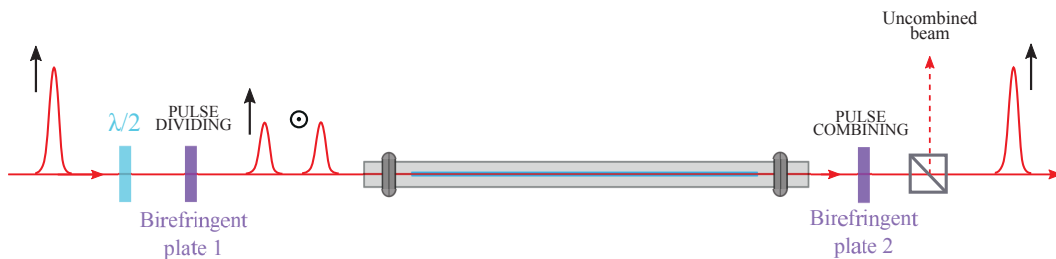
Figure 8.5 – Implementation of temporal pulse dividing in a 'One trip configuration' with two similar birefringent plates.
