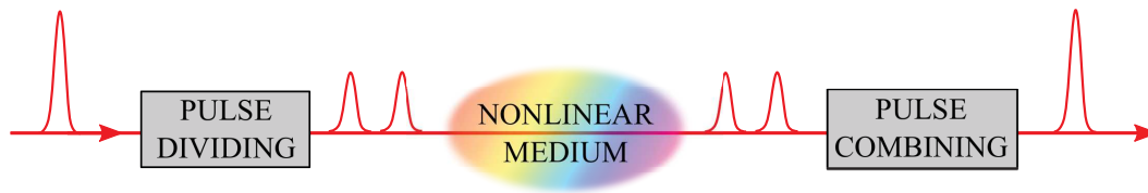
Figure 8.1 – Principle of optical multiplexing.
