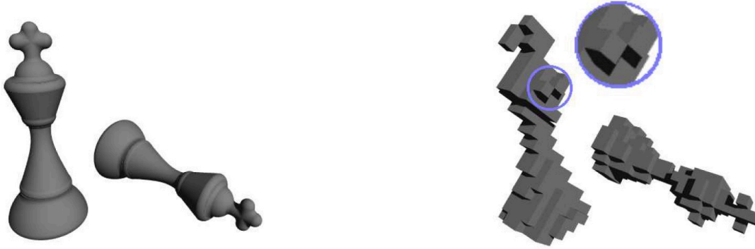
Figure 27.: A reconstruction based on cubical grids in 3D leads to critical configurations [166]
