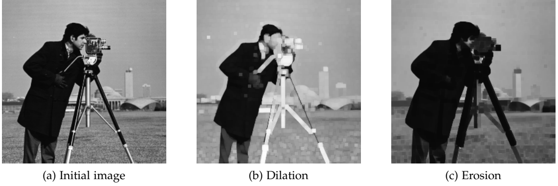
Figure 16: An image (a) and its dilation (b) and erosion (c) by a square of size 4 pixels
