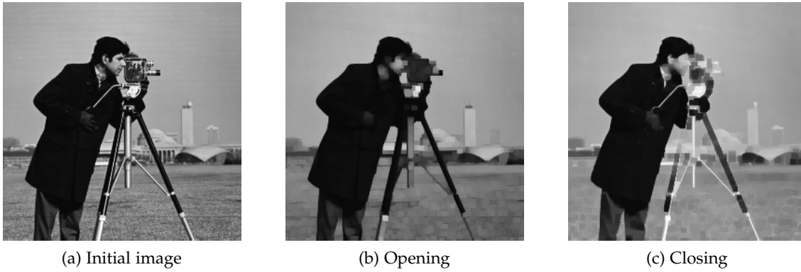
Figure 18: An image (a) and its opening (b) and closing (c) by a square of size 4 pixels
