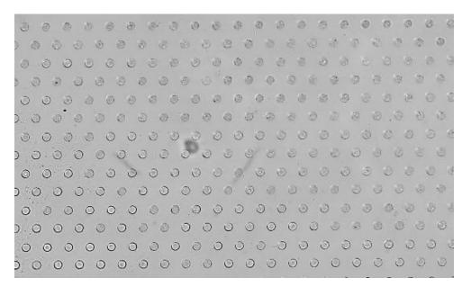
Figure 2 – Microchamber with 500 cylindrical traps with 250  $\mu$ m of diameter by 250  $\mu$ m of height.
