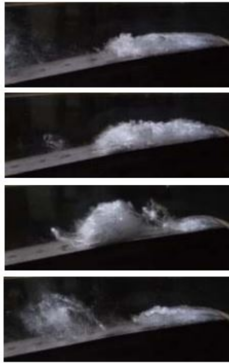
Figure 1.10: Experimentally observed cloud shedding caused by re-entrant jet (taken from [53]).
