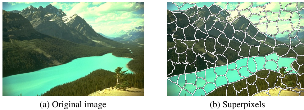
Figure 4.1: Illustration of superpixels (waterpixels)
