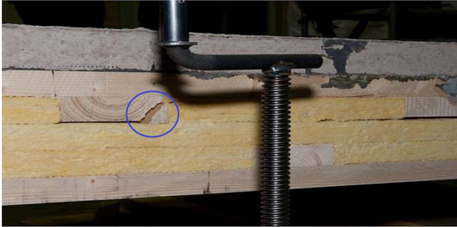
**Fig. 3.6.** Transverse shear cracking (blue circle) between layers 2 and 3 in a transverse wooden strip.
