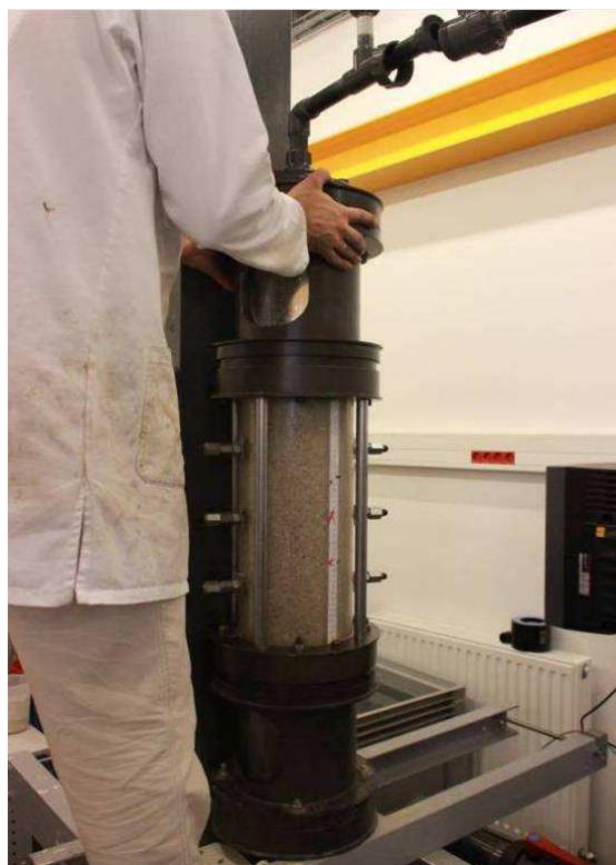
Figure II-38 Installation du cône amont
