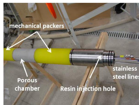
Fig. 1. 14. Measurement chamber of a PP system (from Armand et al. 2015b)
