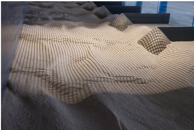
Figure 3.16: Projected grid on dune surface in an experimental configuration with conventionalised groynes. Grid distance is 0.02 m to 0.02 m, picture by Bernd Hentschel (BAW)
