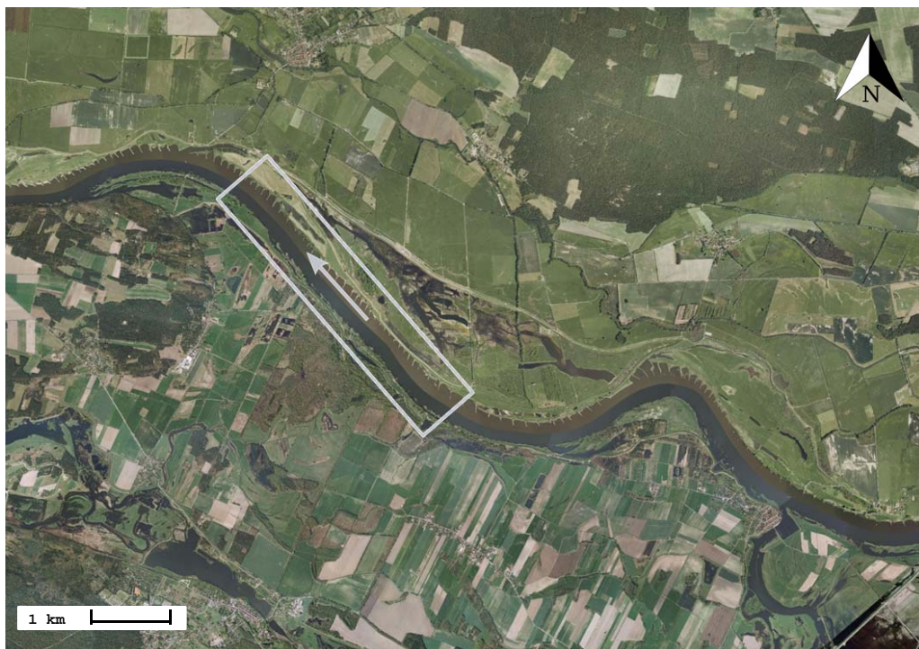
Figure 8.3: Aerial view of evaluated river section of Elbe river; lines mark area of numerical investigation, the arrow indicates the flow direction
