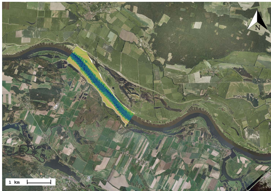
Figure 8.5: Aerial view of the computational domain between El-km 480.0 to 484.0; flood planes behind dikes are not activated at mid water discharge and are therefore not part of computational domain
