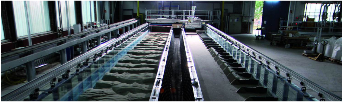
Figure 3.1: Experimental flume for morphodynamic experiments at the Federal Waterways Engineering and Research Institute in Karlsruhe, BAW Bildarchiv
