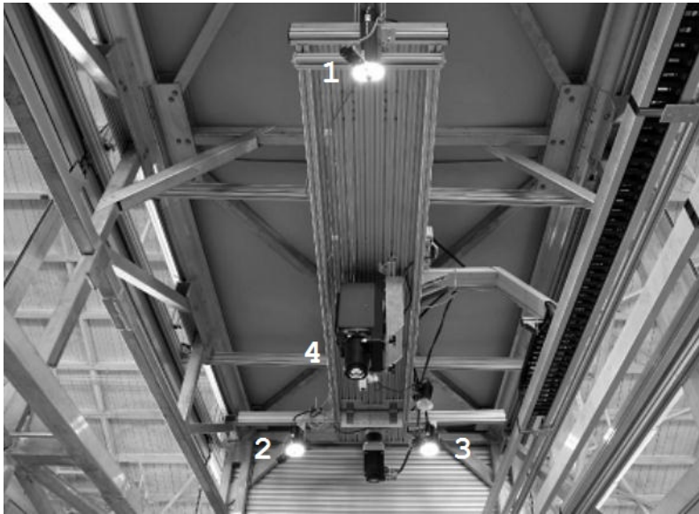
Figure 3.15: Photogrammetric measurement system with cameras with ring-lamps (1–3) and projector (4), picture by Bernd Hentschel (BAW)
