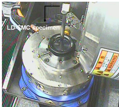
Fig. 1. Experimental setup of X-Ray micro-tomography (EasyTom nano)
