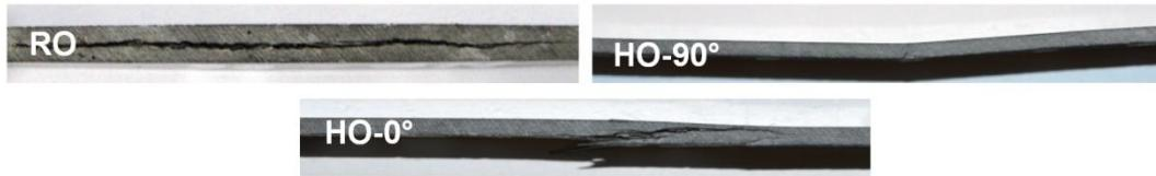
**Fig. 19.** Macroscopic observation of failure surface after compression test
